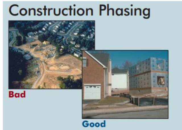
Figure 97. Construction phasing reduces the amount of time soil is exposed (EPA 2003).
