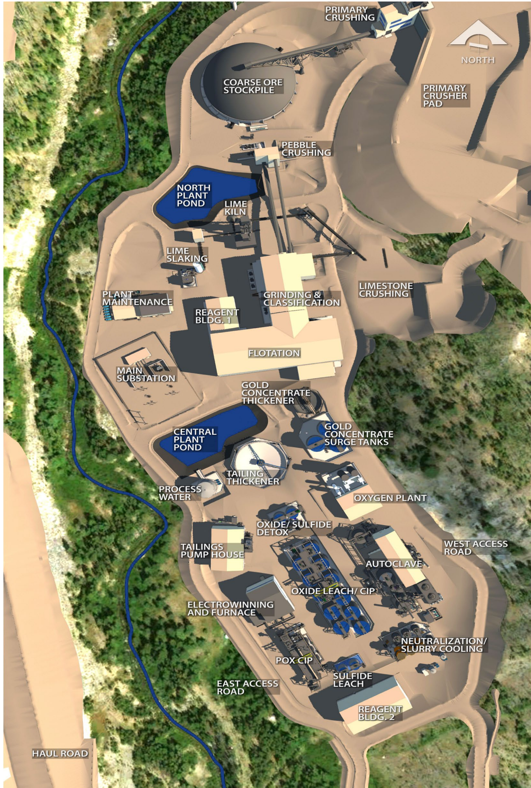
Figure 18-8: Process Area Detail
